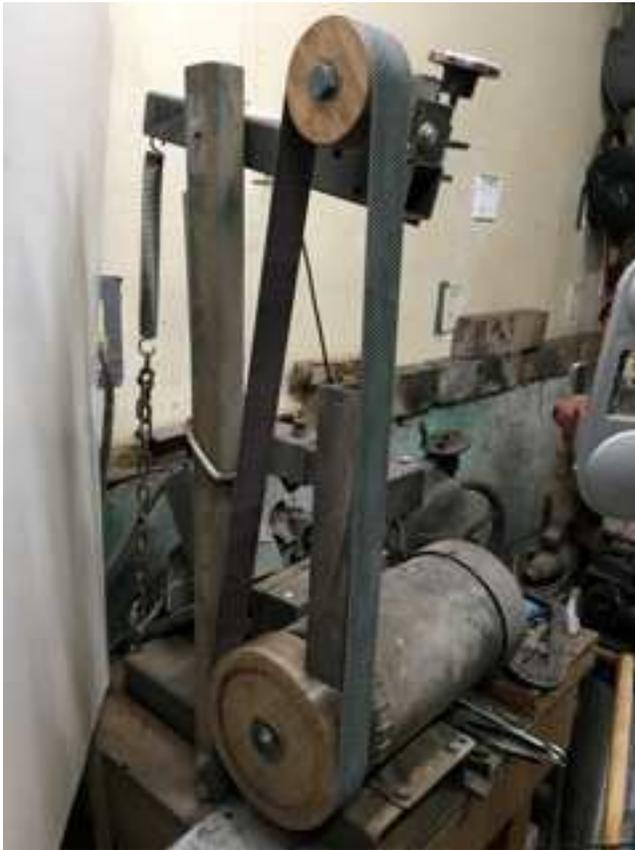
Wayne told me that a two wheel grinder has the most torque. Each additional wheel added to the system reduces the grinder's efficiency. By bolting the frame together rather than welding (not one of my specialties at that time), the frame can be adjusted when it's not aligned.
