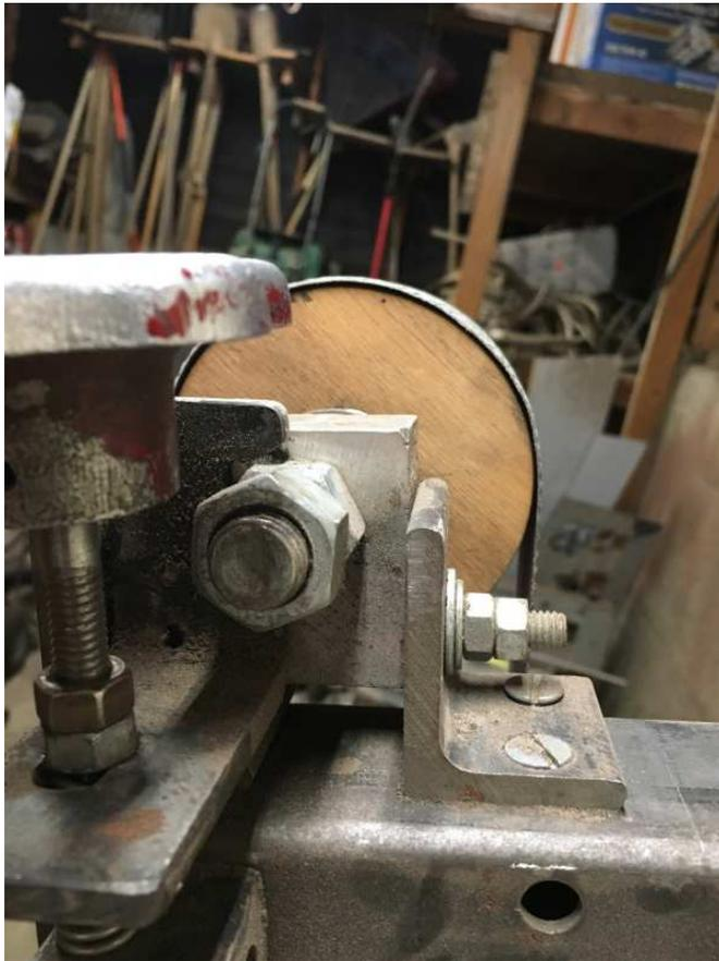
Double nut the end of the 5/8" bolt on the back side of the aluminum block.
