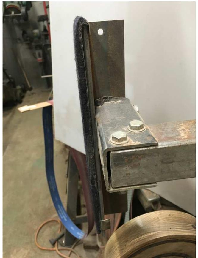
Another different platen attachment is a felt platen. Wayne used a harder felt than I had, but mine seems to work.
