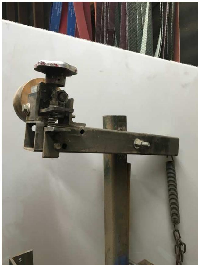
This whole idler/tracking mess is mounted on top of the top pivot arm that is attached to the mast. A strong spring on the end of the top pivot arm gives the tension needed to make the belt keep traction on the drive wheel.
