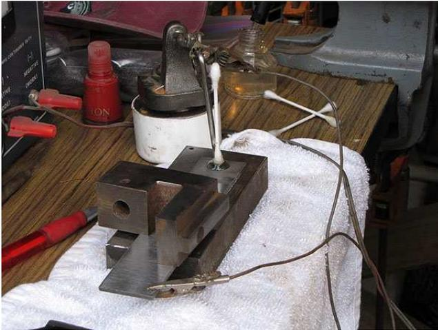
Here's a shot of Wayne's setup with a sample piece of steel that Lynn brought. The Q-tip (being soaked in the saline solution) provides one electrical contact – the other contact is clipped to the “blade”. You can see the puddle of saline solution at the end of the Q-tip. This example is where Wayne used his wax mixture as the “etch resist mask”.
