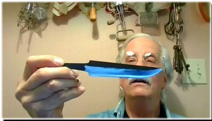
This one is out of heat treat with the edge bevels cleaned up. "It's fairly thin – just under 1/8" – because I pushed the piece I had out quite a bit..." Martin noted that the puukko has a rhombic (diamond) cross section – tapered to the edge and also tapered to the spine.
