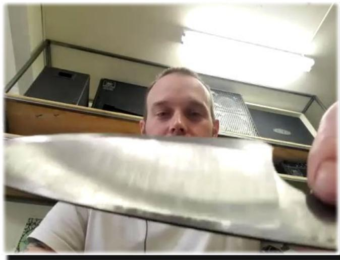
“It's extremely difficult. Do not use a 36 grit belt... Here's a practice run on a broken knife...” Tyler said that a 36” radius platen cuts about 0.025” depth over 1.25” width. He noted that grinding this wide shallow S grind is very difficult to control perfectly.
