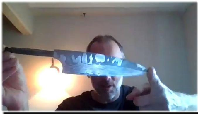
1080/15N20 – a little over 6". "It went OK on the straightening. I had to do about 4 tempers on it [Billy uses an in-the-tempering-oven jig for straightening]."
