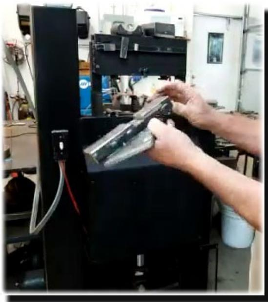
Here's a mild steel test knife. If I understood correctly, he forges the integral knife first, then uses these dies to true it up and set the radiused blade/bolster transition. Then off to the grinder.
