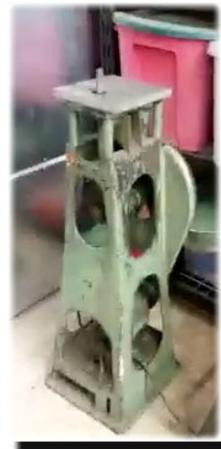
The machine holds a file vertically, using a reciprocating motion. Frank grinds one side of the file smooth so that he can control the cut better.
