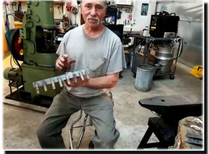
He plans to attach the angle iron to the wall, then hang weights on the end of each Micarta strip, adding 1 lb weights until the strip breaks off the steel.
