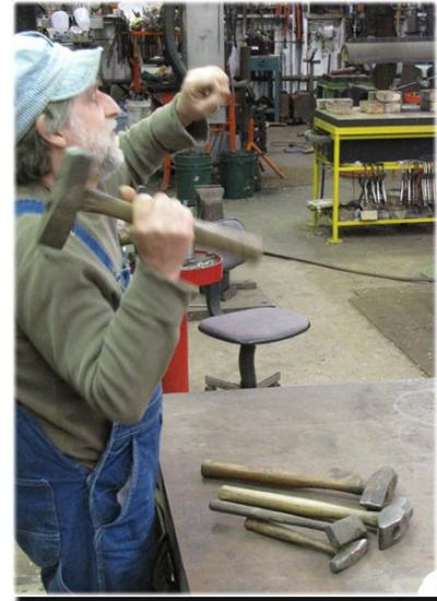
There was discussion about the pedigree and uses of the various hammers. A standard head is great for general shaping. Straight, cross, and diagonal peened hammers are great for moving metal in one direction (at right angle to the peen). Folks have different preferences depending on their forging style and the type of work they are doing. Some folks swear by
