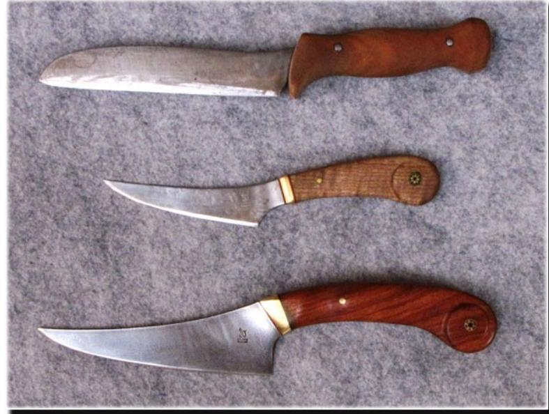
I didn't have a belt grinder yet when I made the old ugly one at top. I'd taken a hunk of modeling clay and squeezed it in my fist as a mock-up for the contours of the handle. It was satisfying to have a knife handle that really fit my hand. I've since gone for a more stylized handle shape – but I've kept some of the contouring of that original handle design so that I'm still happy with how it feels to pick up my knives. And they look a little better IMHO.
