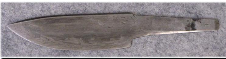
Mike noted that in making cable Damascus he twists it up during the first weld; folds it up and re-twists it during successive weldings; trues it up square before forging a blade from it.
