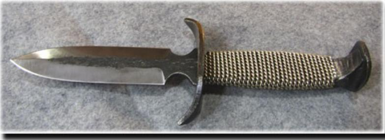
“I wanted to have a guard – but it presented a problem ... how to get the guard on!” So he cut the tang in two – put the guard on – and welded the tang back up before doing the twisted nickle silver wire wrap. Since the piece had already been heat treated he had to wrap the piece up in dripping wet rags while he welded the tang back together.
