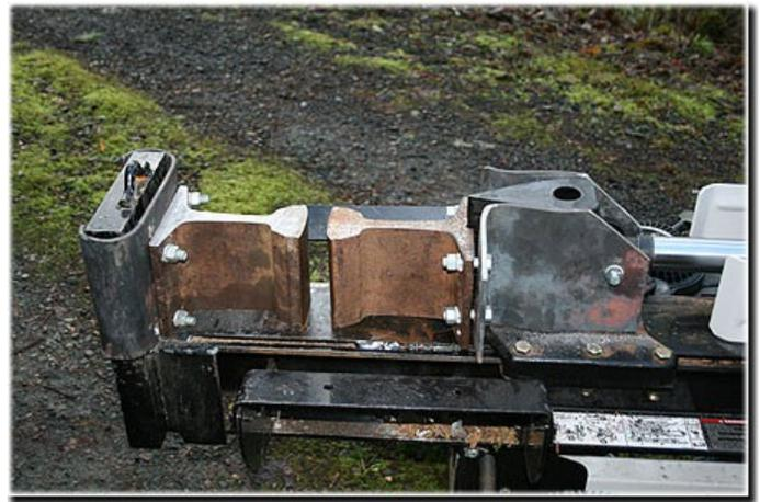
I had to true up the rail faces. And I had to add some brass bushings to the ram head to take some slop out of the action. And it's still kind of sloppy... but hey! I've got a wood splitter and a forge press!
