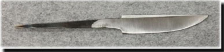
“This was from a grader blade... heat treated in a two brick forge and quenched in Goddard Goop... then I tempered in front of the forge door with a Tempilstik at 350°f.”
