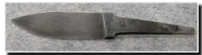
Mike then passed around a dagger he made recently. You can see the temper line on each side. Mike used Wayne's "weenie roast" method for heat treating daggers to get a hard edge and springy center.
