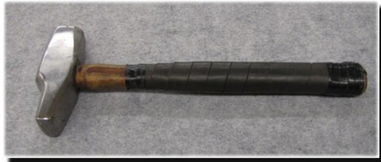
This favorite has a slot down the handle filled with rubber – plus rubber around the outside to reduce vibration (and carpal tunnel). The narrow peen end is good for drawing – the steel moves perpendicular to the peen. For straight-ahead forging, the big end is
