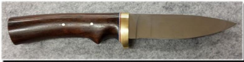
The second knife is his “one-day-knife”. From forging through grinding, heat treat, hafting, and sanded up to 400 grit. To see a photo of the knife after final sanding and finishing, see page 5.
