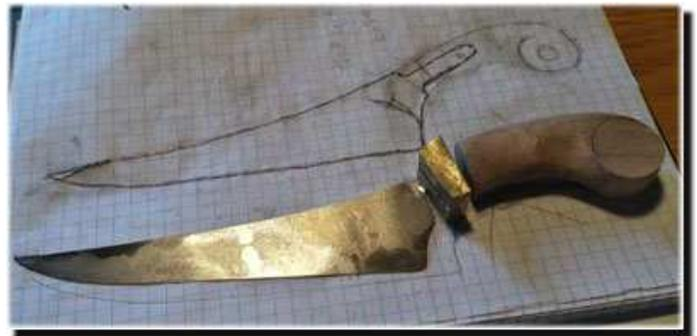
So: toss one in the “oops” drawer and do-over. I'm anxious to try out this chef's knife design – so I have a replacement blade in progress. I'm making the blade from a billet of cable “Damascus” I forged last Fall.
