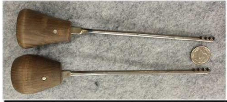
Mike took an old used-up file, ground the teeth off, cut strips out of it, annealed it, cut teeth in it, heat treated it, and put handles on it.
