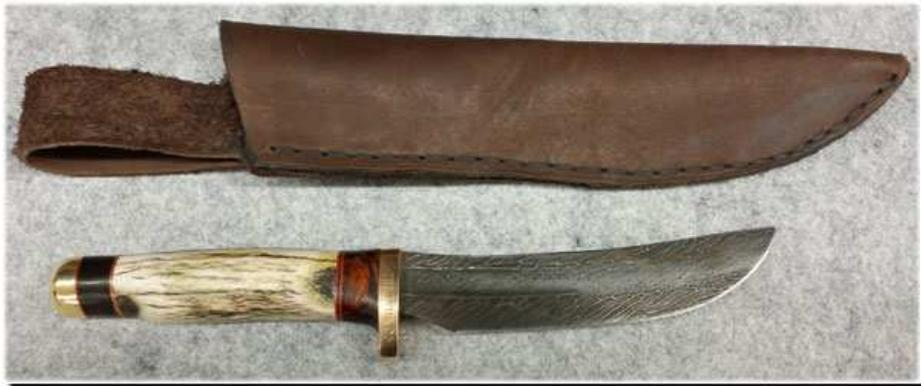
Dan started making Damascus in 1987. He looked Wayne up and Wayne gave him a forge he'd made from a BBQ grill. Dan used it until it burned out – and now uses a propane forge where he makes both pattern welded and wire Damascus.
