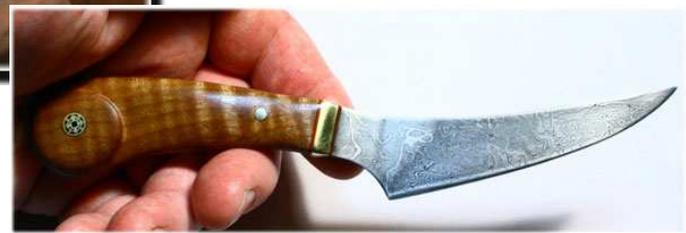
That's 1095/15N20 in the blade (theoretically the billet would have had over a thousand layers – but with all the loss to scale and grinding I'm thinking the blade wound up with one or two hundred layers). That's a maple handle treated with coconut oil, and one of Sally Martin's mosaic pins.
