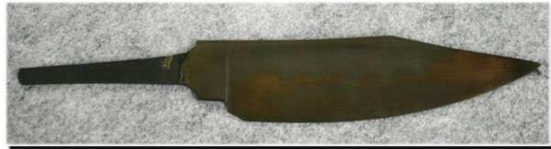
On the smaller knife Mike went ahead and finished it down to 2000 grit and did multiple etches in ferric chloride (with 0000 steel wool rubs between etchings). I got a better photo of this one:
