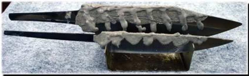
“You have to be sure that the claying is 100% dry – otherwise it's going to bubble up, it's going to blow off, it's going to do many strange and ugly things.” He lets the clay dry for several days. If you try to heat it to dry it the clay will bubble up. When it is truly dry it becomes really hard.
