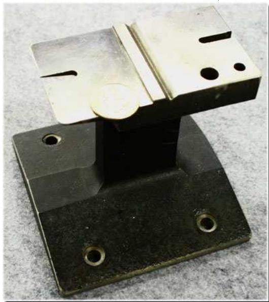
Craig praised and passed around a “Kant Twist” clamp that pinches down without the inevitable twisting you get with a C clamp:
