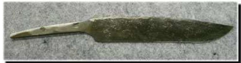
From spark testing and how it works at heat, Martin is wondering if it is an S series steel.
