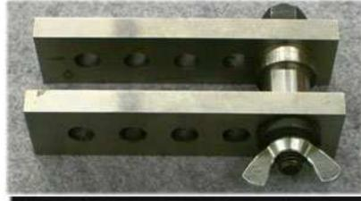
And a set of parallels and a set of 1-2-3 blocks – useful in securing even odd shaped pieces (like antler) for working or drilling.
