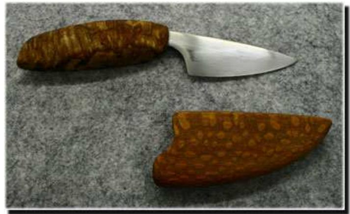
**MARTIN BRANDT** has been working some old rototiller tine into a blade... which can be a bit of a challenge when you have to test-and-guess about steel composition and work around bolt holes and such... but Martin loves working with recovered material.
