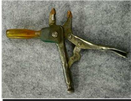
I learned from Wayne to have at least one vice-grip in the shop with copper sheet wrapped around and glued to the jaws (to hold steel without marking it).
