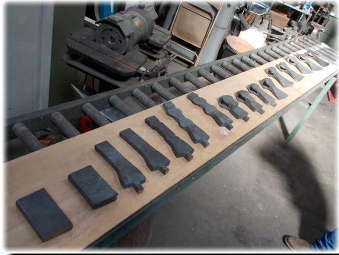
Owen Bush (from the U.K.) demonstrated the construction of a multiple-bar broken-back saex. This was based on an archeological find constructed of eight separate bars of steel welded together, four of them twisted pattern-weld. Plus the wolf-tooth pattern inserts.
