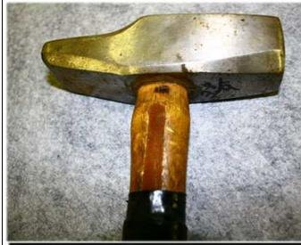
He outlined a couple of options for creating shock absorbing handles – coating with cast-able rubber &/or cutting a groove out of the center of the hammer and filling it with rubber.
