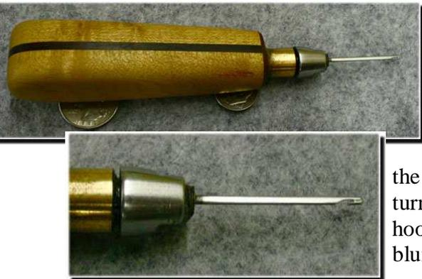
and thinned down the sides. This is used by passing it through the hole empty, then pull the 1<sup>st</sup> thread back through the hole. He set the needle in a nice big wood handle grip:
