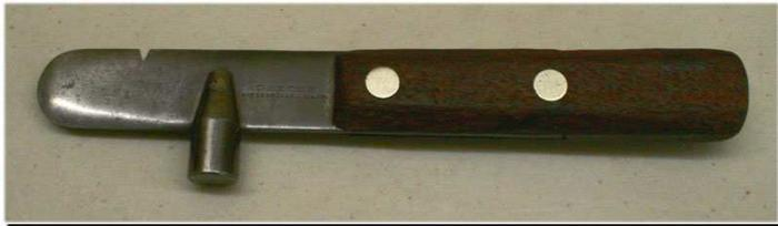
You use the round end to cut the paper seal – the notch to pop the box tacks – and the hammer to close the box back up again!
