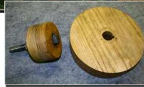
Mike Johnston shared some grinder rebuild he's been doing – making wood parts. The big drive wheel is a couple of pieces of oak laminated with Titebond III – he relayed all his trials and errors getting it sized and trued up. It's never as simple as it first seems. He's running the drive wheel at 1725 RPM. The smaller tracking wheel – set the bolt into the bearing by freezing
