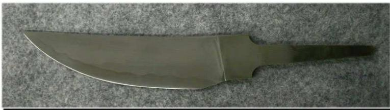
Mike applied a thin layer to the main part of the blade – leaving the edge without clay. Unlike the Japanese method, there was no thick clay layer.
