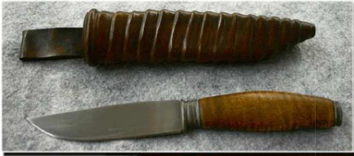
show through the stone washed surface. Ray asked where Ben stops on grit before tumbling, and Ben feels that if you take it up to 220 you should be fine. Ben etches in Ferric Chloride first, then tumbles the blade. On the blue handled blade Ben wiped it down afterward with cold bluing.
