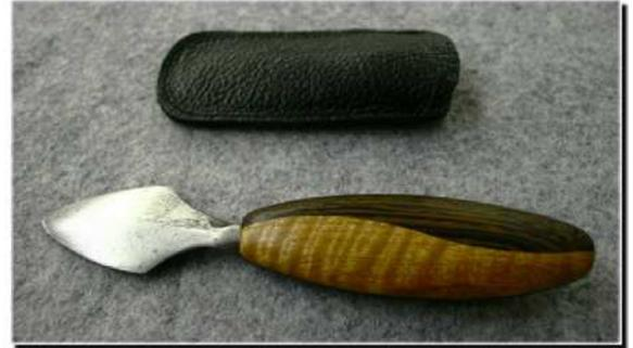
Mike Johnson passed around a knife made from coil spring and a piece of unknown wood (Padauk?) and a clip point "that's been fighting me for awhile":
