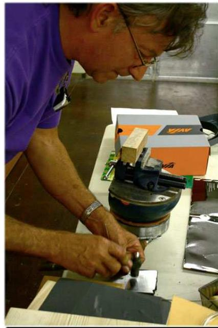
To set wire into the cut slot, bend the wire to the shape of the slot and cut to length. If this wire goes to the end of a line – or one end of it lays next to another wire – you might hammer or sand that end of the wire flat so that it blends smoothly rather than with a square shoulder.
