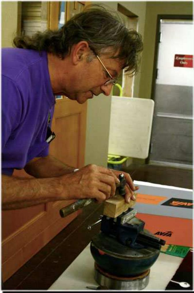
You might notice in the above photo that the wood is held on top of the vice jaws by metal knobs that Wayne set into the top of the vice. Two on one jaw and one on the other. This configuration allows firm gripping of non-rectangular pieces.
