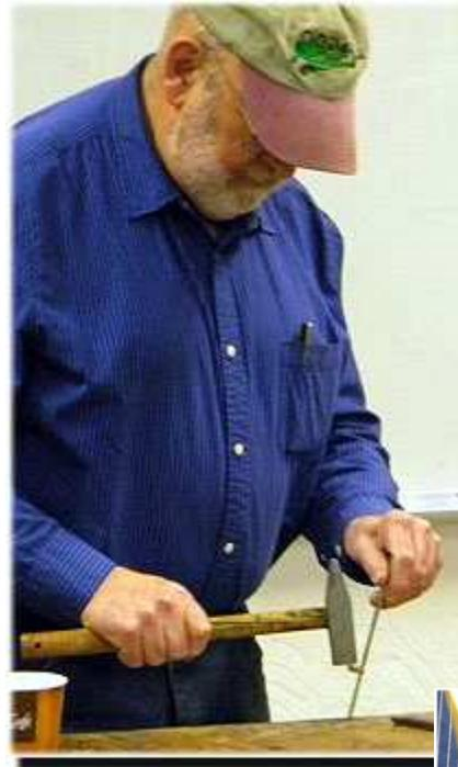
To demonstrate the strength of the solder Wayne started hammering on the guard to break the joint. After several attempts to knock off the guard, Wayne put the blade in a vise and continued striking the guard with a small cross peen hammer several times before the joint failed. Wayne
