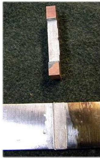
Examination of the joint showed an even and complete coating of silver solder on both the guard and blade.
