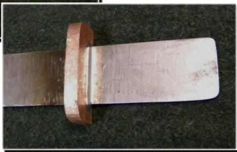
applying solder from a stick or wire. Wayne said he had placed a little too many “snippets” of silver solder on the tang side of the knife as there was a little too much flow through. The amount of excess solder on this joint was far less than most of my joints were AFTER I cleaned them up.
